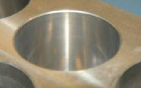
Good lubrication from Castrol® Alusol® produces a high-quality finish, 0.1 Ra (Roughness average) for precision components
