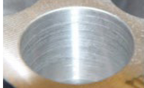
Poor lubrication reduces surface finish, 0.8 Ra, and can lead to parts being rejected
