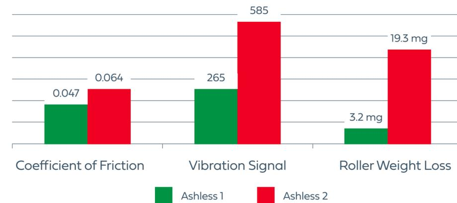
The Castrol product demonstrated a lower coefficient of friction and registered a significantly lower vibration signal, while demonstrating excellent performance in controlling wear as evidenced by lower roller weight loss.
